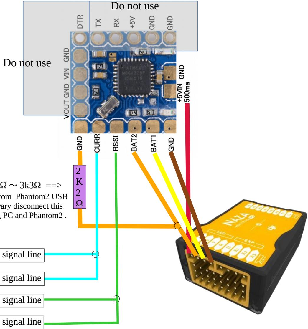
Resistor about  $1k\Omega \sim 3k3\Omega$  ==>
