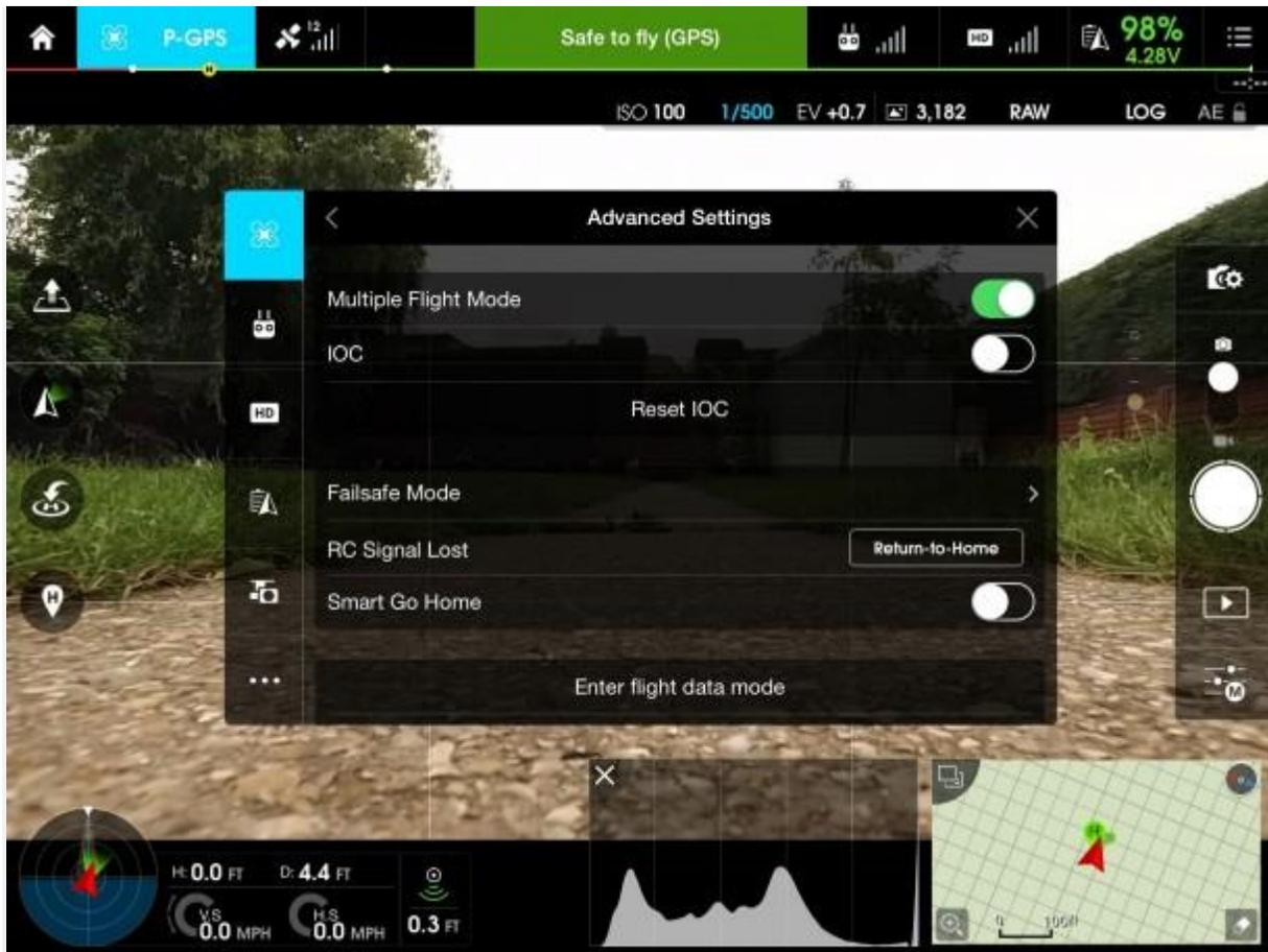
In the image above note the option called “Multiple Flight Mode”. With Multiple Flight Mode enabled you can now switch to ATTI mode using the mode switch on the controller. Flying in ATTI is not that different from flying in GPS mode: the drone will still maintain its altitude and the controls still function the same. The main difference is that the drone will no longer hold position automatically, it will be affected by any wind as well as its own inertia.
