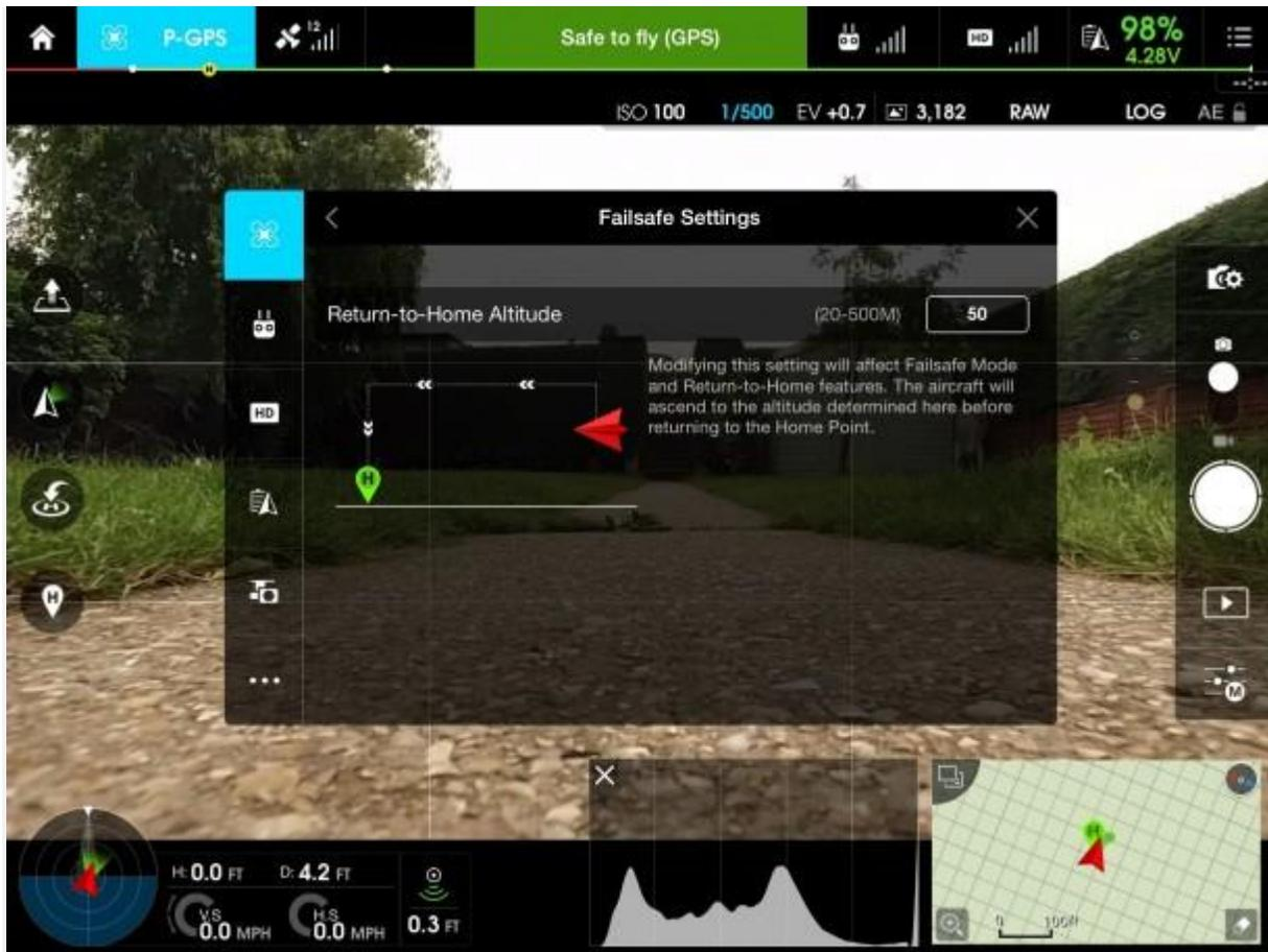
It's also important to check that the correct home point has been set for each flight. When the motors start there should be an audio alert saying "The home point has been updated, please check it on the map", it's worth doing that just to make sure the home point is where it should be.
