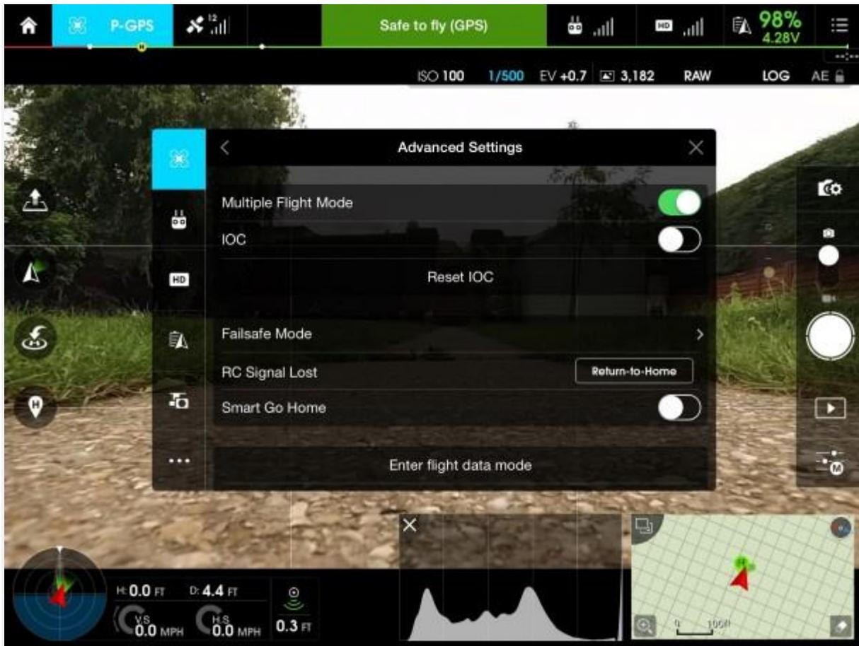
By disabling this option the drone will simply initiate a landing at its current location rather than head home once it reaches 10% power. As always though you need to make the call with each flight, as there could be times when it's better to leave Smart Go-Home enabled. The Go app also monitors the power required to get the aircraft back to the home point and will initiate a return to home automatically if Smart Go-Home is enabled.
