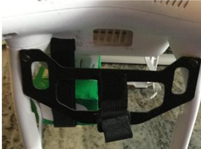
Secure under the VPS: This method is usually used when flying with one, single larger sized battery. You secure the battery under the VPS of the aircraft. Some use dual lock by 3M, some use industrial strength Velcro and some use straps, as shown below. Dual lock is recommended, but make sure its secure no matter what you use!
