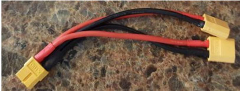
XT60 Dual Adapter: This adapter does not include the wire, is more hard wired of just some male/female xt60 plugs. This is usually the less heavy option.
