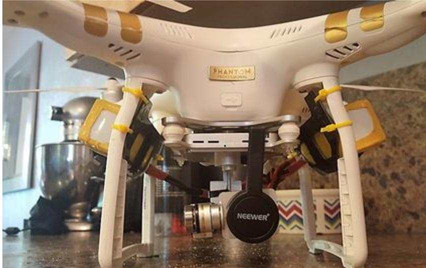
Rationale: The main reason for adding additional batteries to your Phantom 3 is to extend the time of flight available in the air. This could be to achieve longer flight distances, record more video, get to that special remote spot to take a sunset picture or just a failsafe to the stock battery.
