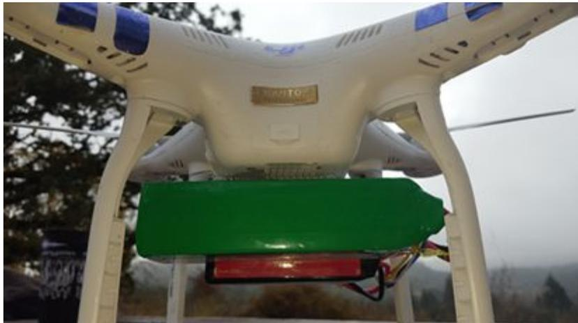
Dual small battery: This is where you would take two smaller batteries and add them together using an adapter for the two. This would usually be 2x1800mah, 2x2300mah or 2x2800 mah. Common examples are Turnigy Zippy Compact 1800, Venom Fly 2300 or Maxamps 2800. Note, if you use two at a time, you will need an adapter.
