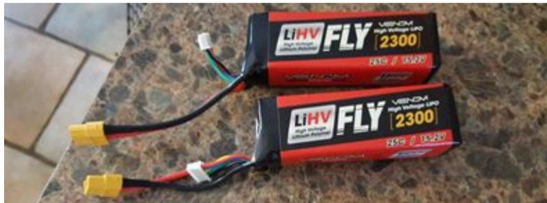
Split big battery: This is where a single big battery (usually Multistar 5200 or 6600) are split into a pair of battery packs, to fit on the battery trays on the landing gear. Such as below:
